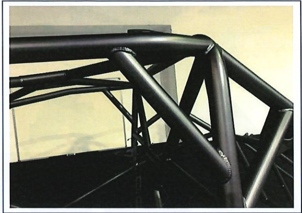
PHOTO 8 MAIN ROLLBAR TO "B" PILLAR ATTACHMENT
