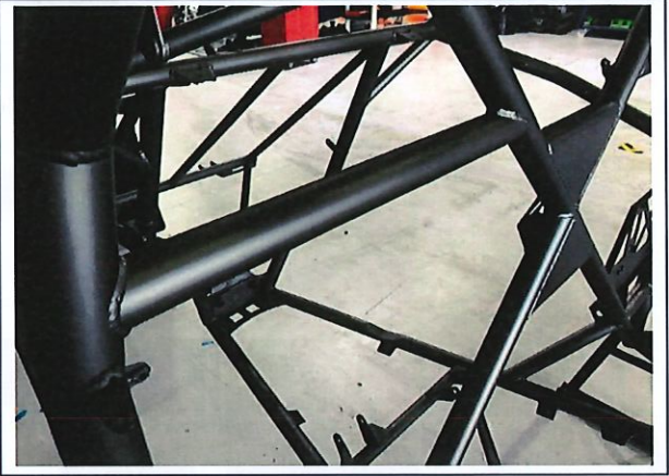
PHOTO 13 SHOULDER HARNESS ATTACHMENT – CO-DRIVER
