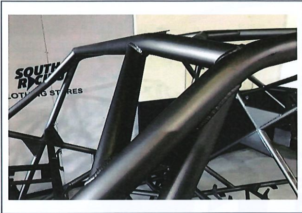
PHOTO 7 FRONT ROLLBAR TO "A" PILLAR ATTACHMENT
