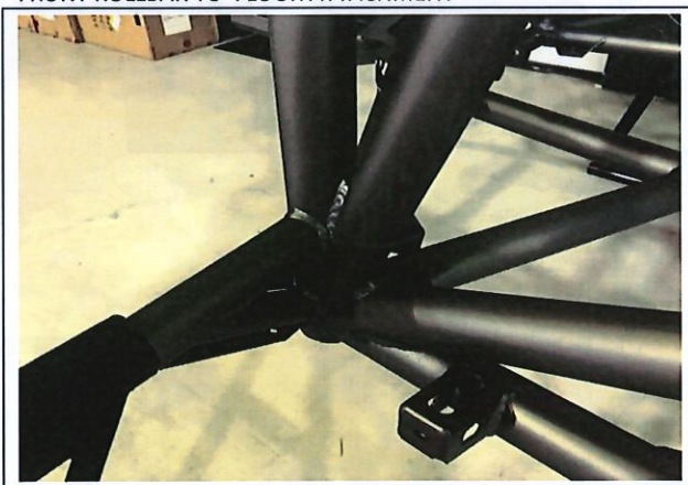
PHOTO 6 FRONT ROLLBAR TO FLOOR ATTACHMENT
