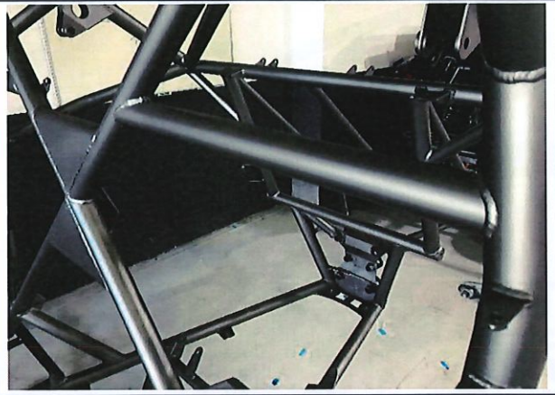
PHOTO 12 SHOULDER HARNESS ATTACHMENT – DRIVER
