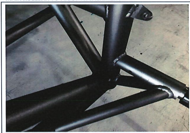
PHOTO 4 MAIN ROLLBAR TO FLOOR ATTACHMENT
