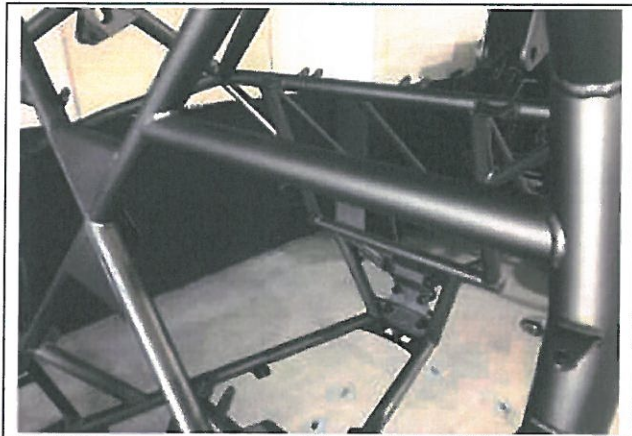
PHOTO 12 SHOULDER HARNESS ATTACHMENT – DRIVER
