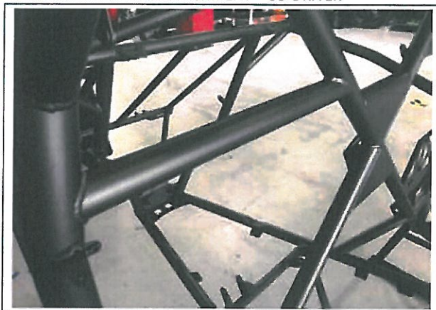
PHOTO 13 SHOULDER HARNESS ATTACHMENT – CO-DRIVER
