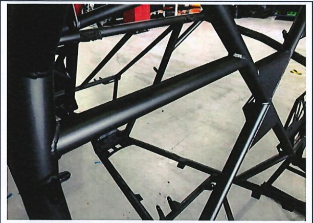
PHOTO 13 SHOULDER HARNESS ATTACHMENT – CO-DRIVER
