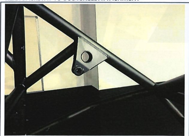
PHOTO 5 REAR BACKSTAY TO BODYSHELL ATTACHMENT
