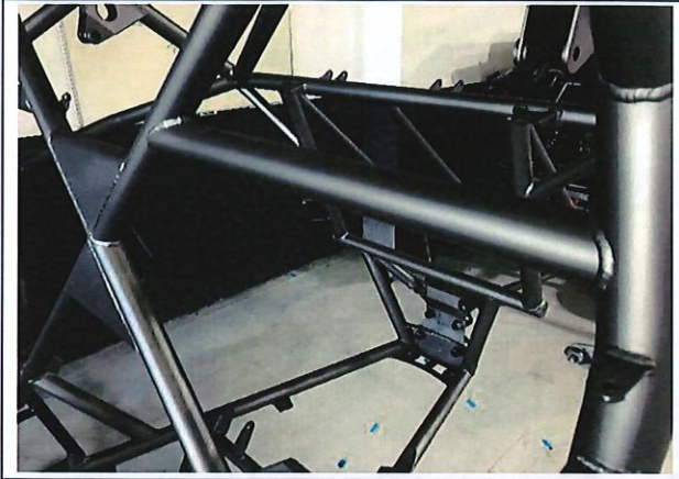
PHOTO 12 SHOULDER HARNESS ATTACHMENT – DRIVER
