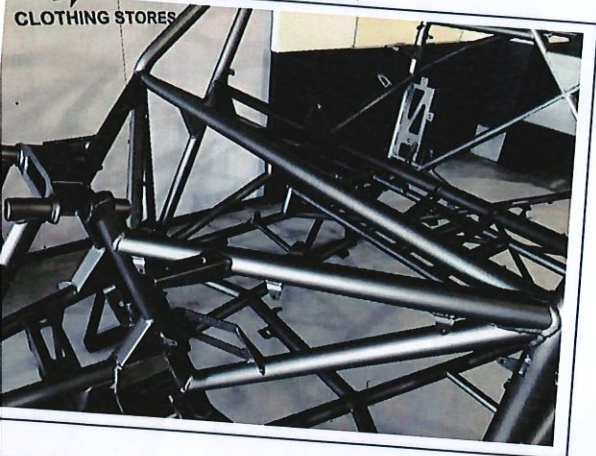
PHOTO 10 ANTI-INTRUSION DOORBAR - DRIVER
