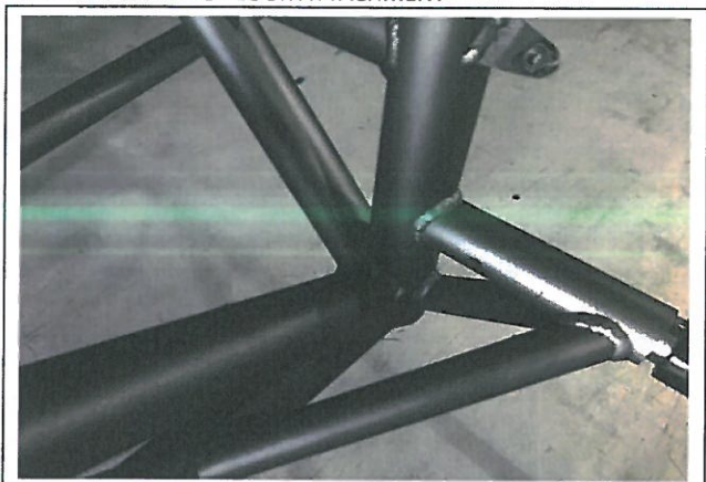
PHOTO 4 MAIN ROLLBAR TO FLOOR ATTACHMENT
