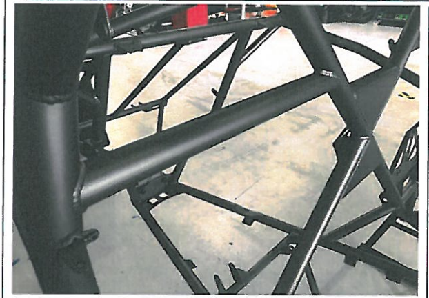
PHOTO 13 SHOULDER HARNESS ATTACHMENT – CO-DRIVER
