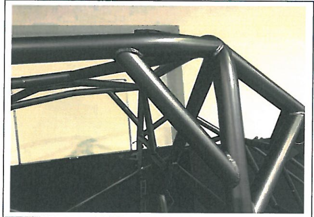
PHOTO 8 MAIN ROLLBAR TO "B" PILLAR ATTACHMENT
