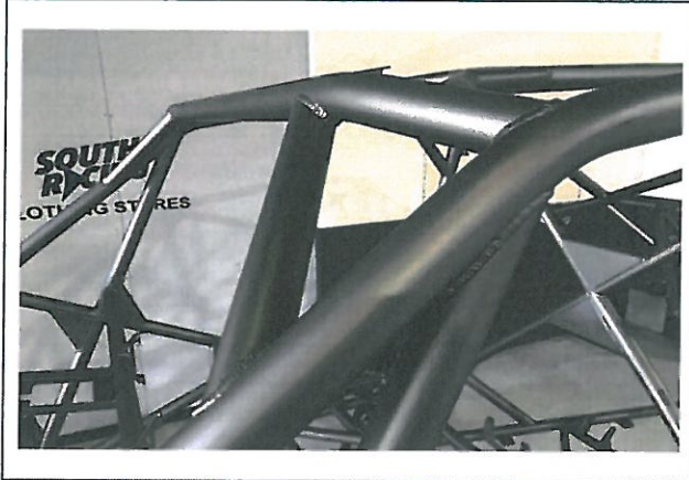
PHOTO 7 FRONT ROLLBAR TO "A" PILLAR ATTACHMENT
