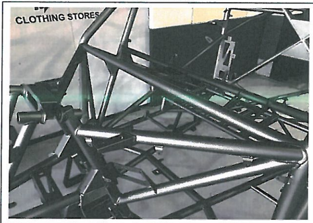
PHOTO 9 ATTACHMENT TO FRONT SUSPENSION
