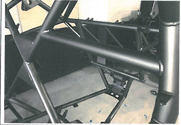
PHOTO 12 SHOULDER HARNESS ATTACHMENT – DRIVER
