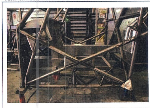
PHOTO 10 ANTI-INTRUSION DOORBAR - DRIVER
