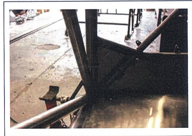
PHOTO 6 FRONT ROLLBAR TO FLOOR ATTACHMENT
