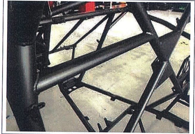
PHOTO 13 SHOULDER HARNESS ATTACHMENT – CO-DRIVER
