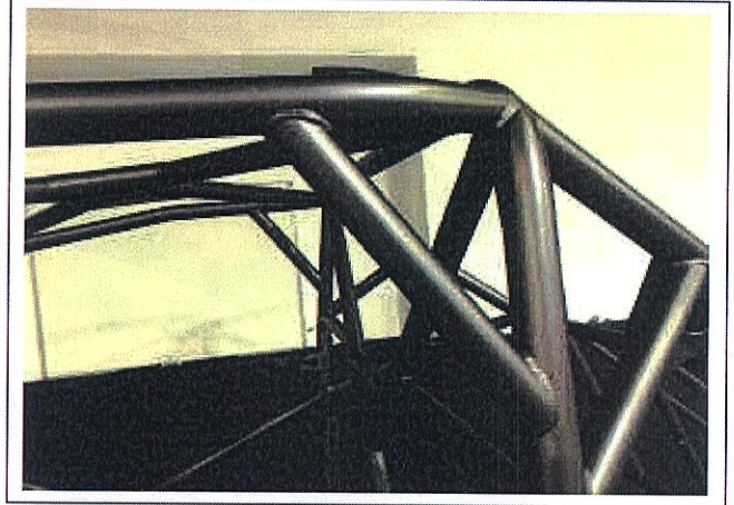
PHOTO 8 MAIN ROLLBAR TO "B" PILLAR ATTACHMENT
