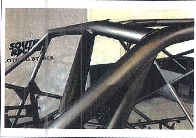
PHOTO 7 FRONT ROLLBAR TO "A" PILLAR ATTACHMENT
