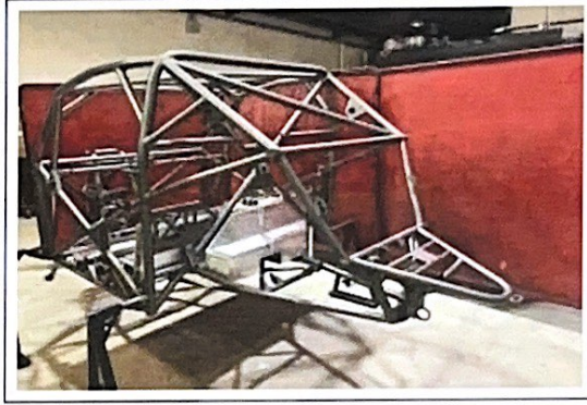
PHOTO 4 MAIN ROLLBAR TO FLOOR ATTACHMENT
